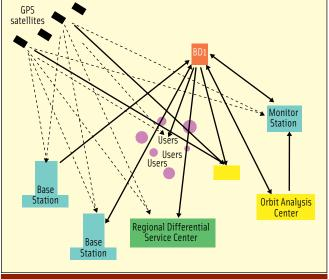
FIGURE 8 Augmentation scheme based on Beidou satellites
